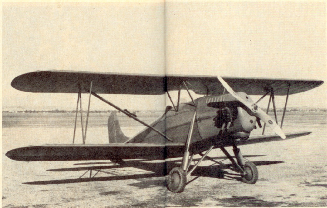
The production Rose A-1 Parrakeet of 1934. Since the Parrakeets were not delivered with airspeed indicators, the owner of this one installed an old-fashioned vane-type instrument on the diagonal strut. A.U. Schmidt photo.
